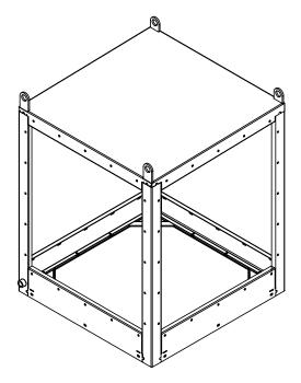
For side inlet fans, remove panel at end of plenum. This opening is the designed connection spot for user connected ductwork from building.
